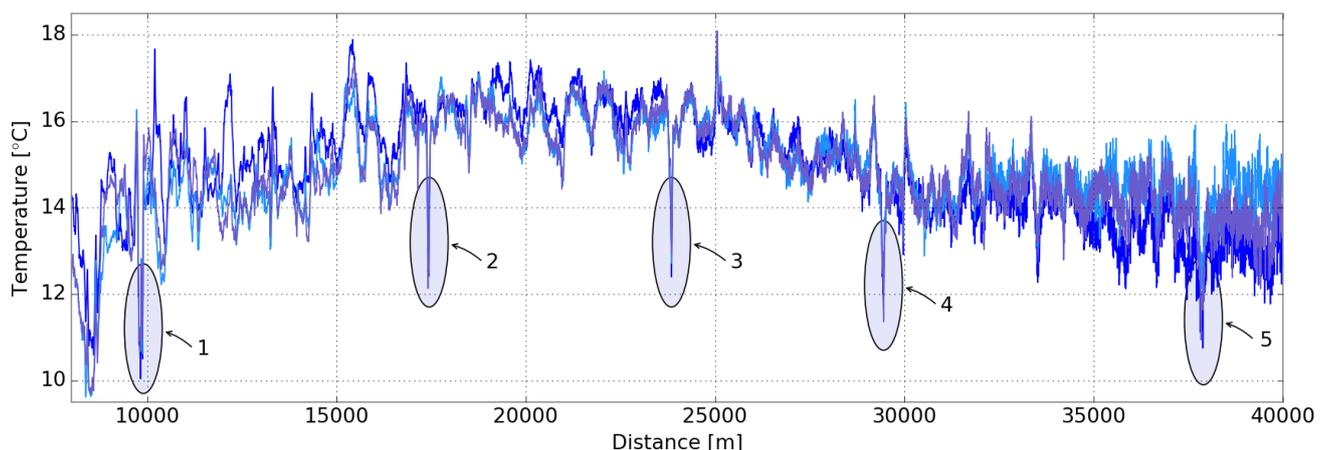
Fig. 3: DTS traces before cable reburial with five identifiable cold spots
